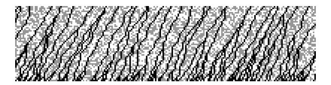
Figure 2.6: Automaton performing random walks iterated on the uniform measure.  $\blacksquare$  is a particle, while the second layer is represented by  $\square$  (0) or  $\blacksquare$  (1).
