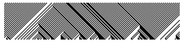
Figure 0.4: Space-time diagram of the traffic automaton from an initial configuration drawn uniformly at random.
